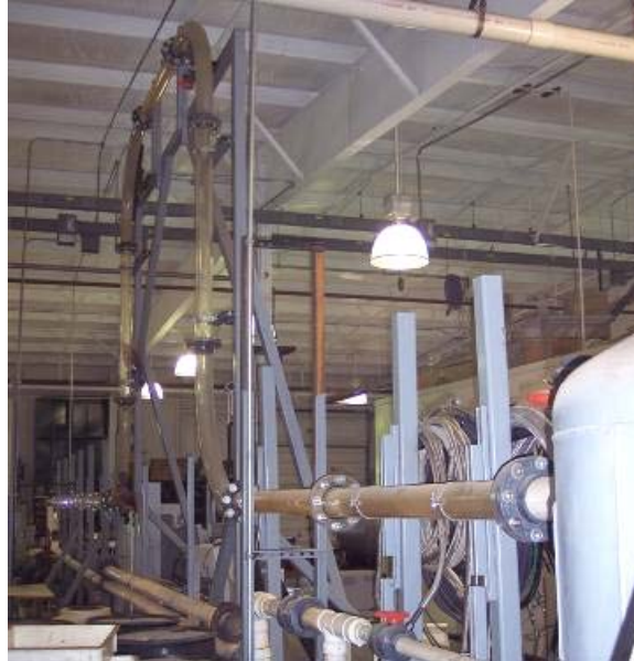
Figure 11: Picture of the inclined section of the transparent hilly terrain flow loop
