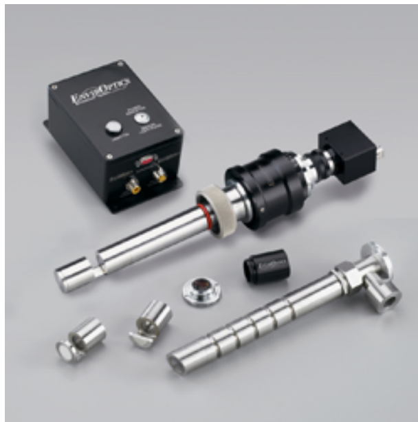
Figure 4: In-situ video camera for live observation of corrosion phenomena (org.: envirotec.com)
