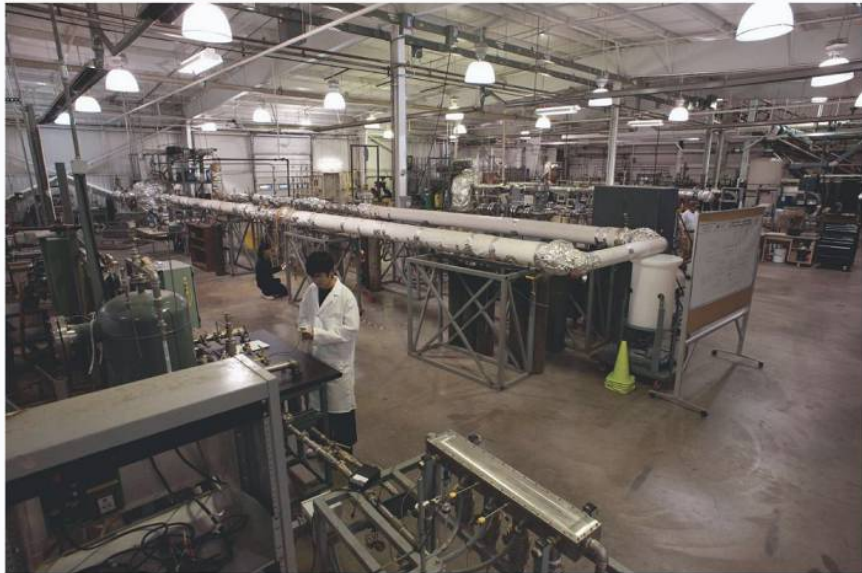
OU graduate students check the operation of the 30-m long wet gas corrosion flow loop, which is designed to study the corrosion effects of operating parameters on CS under dewing conditions during the transportation of wet gas. Photo copyright Gary J. Kirksey 2010.
