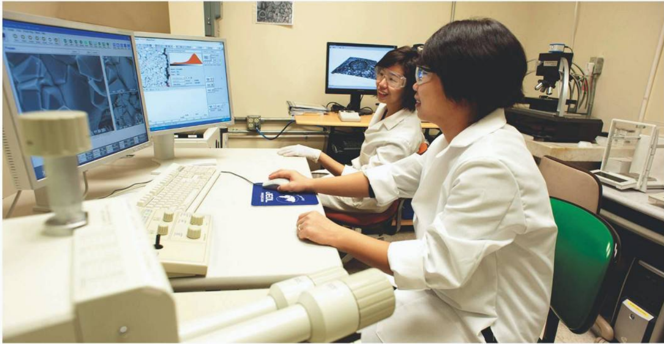
Ph.D. students Yang Yang (front) and Kod Pojtanabuntoeng analyze the surface of a corroded CS sample using a scanning electron microscope (SEM) and an optical infinite focus microscope (IFM). Photo copyright Gary J. Kirksey 2010.
